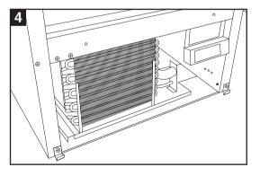
**4.** The condenser coil fins are now accessible for cleaning.
