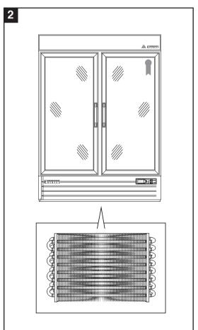
2. The condenser coil is behind the vented grill at the bottom of the unit.
