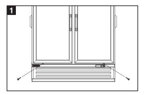
1. Remove two screws from the top of the vented grill.
