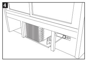
**4.** The condenser coil fins are now accessible for cleaning.
