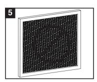
5. Do not attach an aftermarket filter or screen around the condenser coil. This obstructs ventilation which leads to overheating, component failure or the risk of fire.
