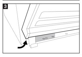
3. Lift the vented grill vertically until the two keyholes on its bottom edge clears the stationary bolts.
