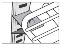
Place shelves on the shelf clips making sure all corners are mounted securely and evenly with identical distance from the unit's floor and up. Always lay the back of each shelf down on the rear clips before the front.
