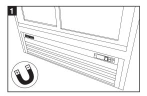
**1.** The top of the vented grill is held in place by magnets.
