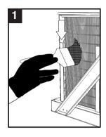
Use a long bristled brush in a vertical sweeping motion to remove lint, dust and debris from in between the metal fins of the condenser coil. Do not apply heavy pressure so as not to bend the fins.
