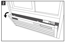
**2.** Lightly pull on the top edge of the vented grill so that it swings open a quarter of the way.
