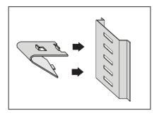
Attach the shelf clips onto the pilasters by inserting its top hook into a pilaster notch followed by the bottom hook. Do not use pliers or other crimping tools to modify the shape of the shelf clips. This will result in shelf mounting instability.
