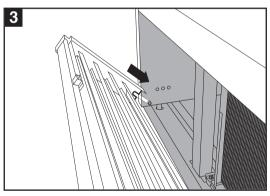
**3.** Lift the vented grill vertically until the two keyholes on its bottom edge clears the stationary bolts.
