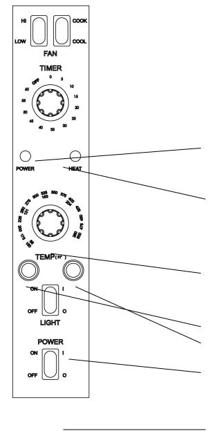
thermostat related problems could be attributed to their being out of adjustment (calibration). Athermostat that is out of calibration may cause unsatisfactory cooking results such as uneven baking, prolonged cooking times, etc. If you are experiencing uneven cooking, it may be a result of excessive cooking temperatures. Refer to the cooking chart provided in Operating Instructions Section C.
