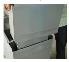
4. Secure it with four self-tapping screws two on the back and one on each side using a 5/16" socket
