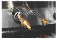
Replace the orifice fittings into the valve.
