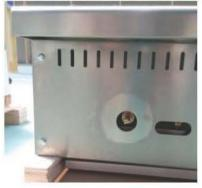
2. Unscrew bolts and pilot valve, then remove manifold.
