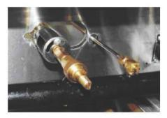
Replace the orifice fittings into the valve.
