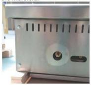
2. Unscrew bolts and pilot valve, then remove
