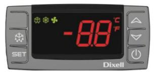
**SET**: To display target set point; in programming mode it selects a parameter or confirm an
