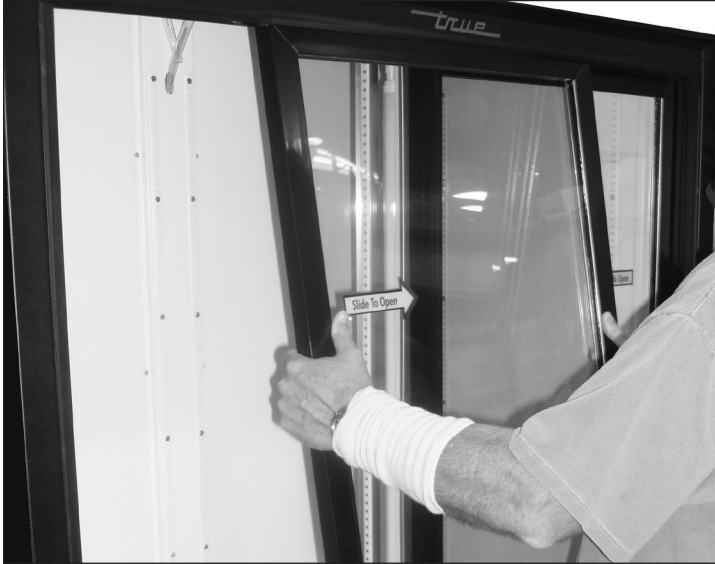
Fig. 4. Carefully remove the door.
