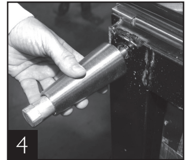
4 Thread leg into cabinet bottom frame rail.
